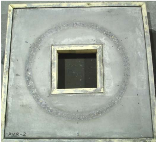
Fig. 2: Left - AVR-2 Abraded Wear Track Plan, Right – Abraded Wear Track Profile Close-up.
