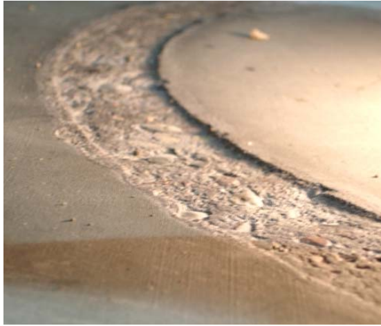
Fig. 2: Left - AVR-2 Abraded Wear Track Plan, Right – Abraded Wear Track Profile Close-up.
