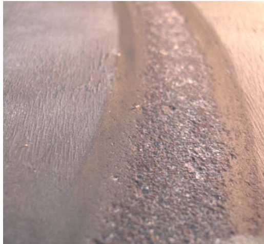
Fig. 3: Left - AVR-1 Abraded Wear Track Plan, Right – Abraded Wear Track Profile Close-up.
